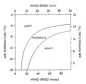
Icing conditions for vessels heading into or abeam of the wind for water temperatures of  $+7^{\circ}\text{C}$  (45°F)
