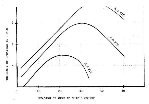
Figure 1-23 AMOUNT OF SPRAYING VERSUS HEADING OF SHIP TO WAVE
