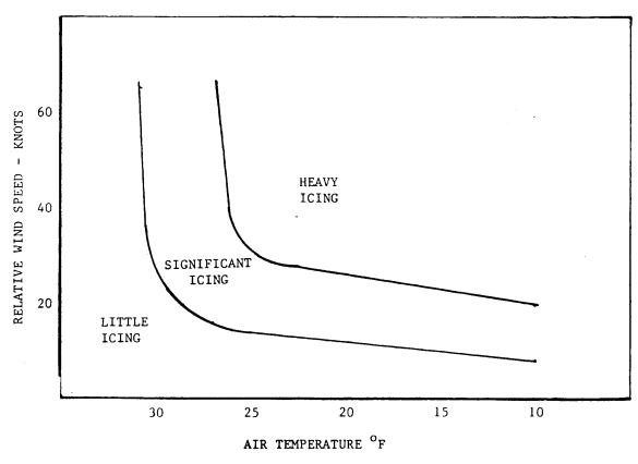
Figure 1-24 WIND SPEED VERSUS TEMPERATURE
