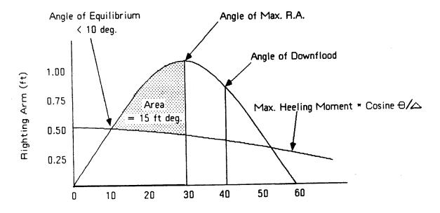
Figure 1-7. Lifting Criteria
