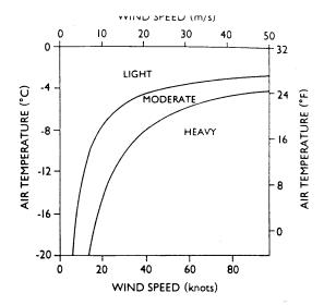
Icing conditions for vessels heading into or abeam of the wind for water temperatures of  $+3^{\circ}C$  (37°F)
