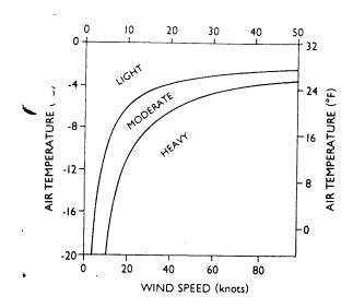
Icing conditions for vessels heading into or abeam of the wind for water temperatures of  $+\,1^{\circ}\text{C}$  (34°F)
